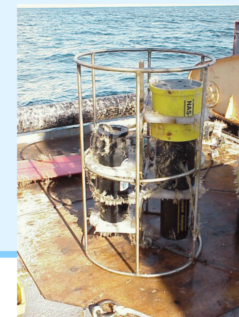
Automated nutrient analyzer clogged up with hydroids
